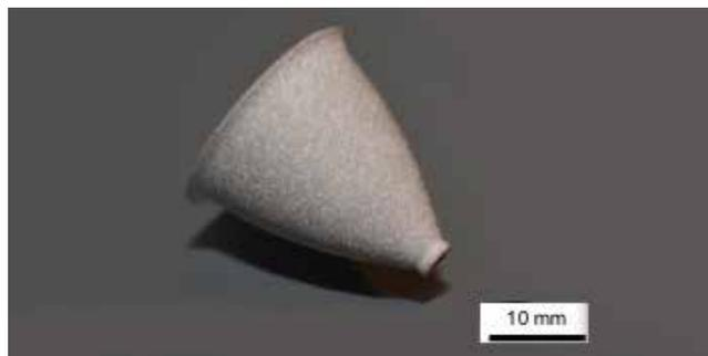
Figure 5: Sintered bell-shaped diffuser made of 316L stainless steel
