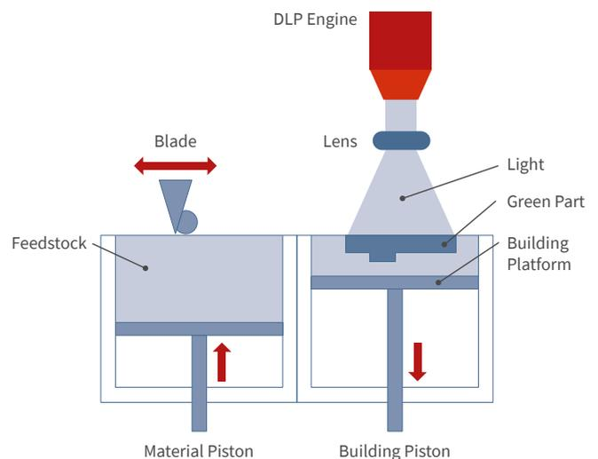
Figure 2: Description of the LMM process
