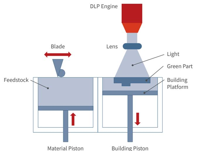
Figure 2: Description of the LMM process
