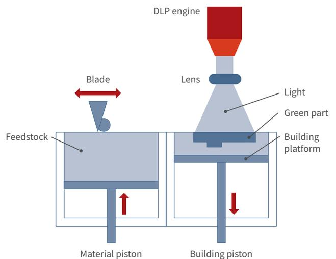
Figure 2: Description of the LMM process
